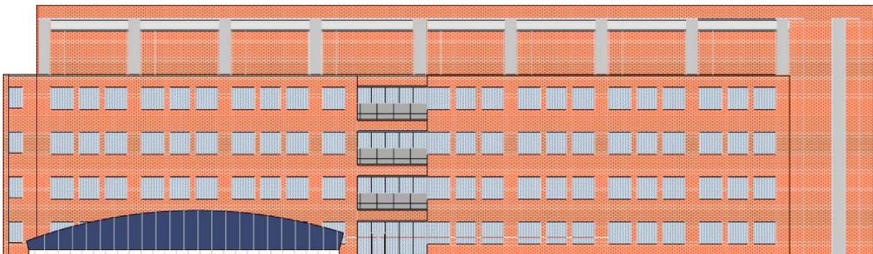
The new elevation takes many cues from the surrounding buildings. The upper level aluminum columns break up the extensive amount of blank brickwork that is needed around the 25' penthouse. The ribbon windows are broken up to reflect the traditional window pattern found in an office building. The cast stone balconies work with this traditional façade just as well as with the modern façade, and provide a look of significance for the entrance.
