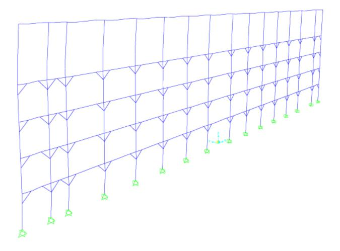
Again, 60 moment connection will be needed at the penthouse level. Below is displayed the displacement of this system as compared to the allowed values of the h/400 criteria.
