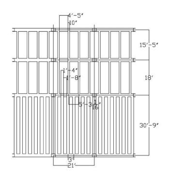
The typical beam is 19.7" wide by 20.5" deep and spans 21'. The reinforcement at the
