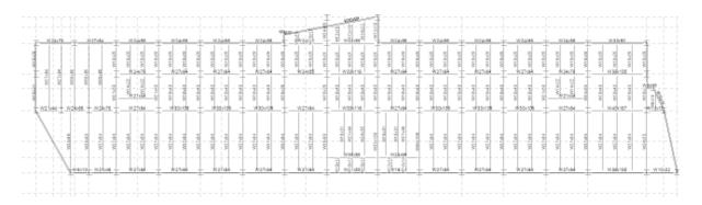
The average beam member sizes came out to be very small due to the small spans with the typical member being a W8X10. However, with longer spans and a great deal of loading from the joist members the girdgers are very large, with the typical member being a W40X167. The typical beam and girder layout and sizes can be seen on the next page.
