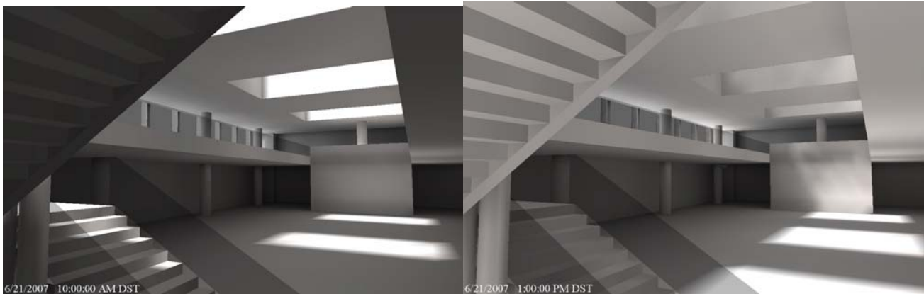
Figure 1.8 – Daylight Study – June, 21 - 10:00 AM & 1:00 PM
