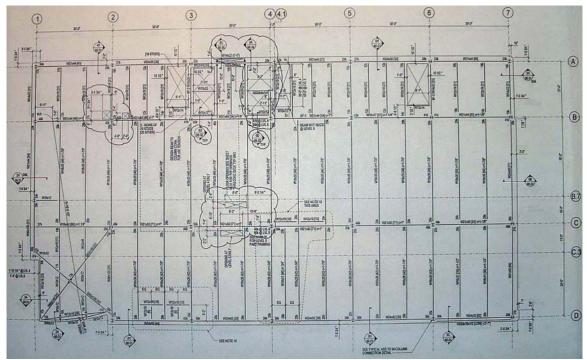
The roof is framed out in the same way the floors are except that none of the roof shapes are cambered. The roof girders range from a W21x44 to a W24x62 while the beams range from W16X26 to W18x40. The high roof framing for the glass/aluminum corner is more simplified than the floor framing and composes of W14 and smaller shapes.
