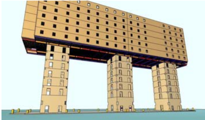
Figure 7 - Observe the multitude of openings in the concrete cores
