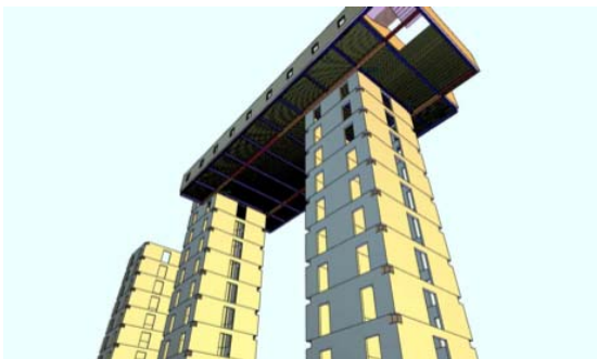
Figure 2 - Half a floor lifted into place
